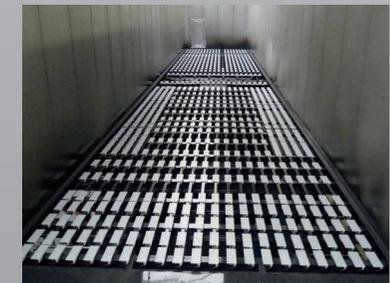
Floor assembly with full-length longitudinal reinforcement
