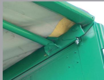
Lifting rear crossbeam (standard variant)
