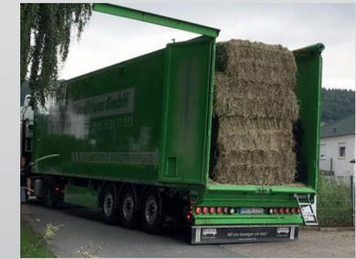
Hinged crossbeam for unobstructed access or crane loading (optional)
