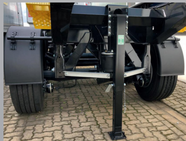
Center landing leg rated for unladen trailer
