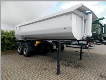
2-axle semitrailer with drop-down landing legs rated for laden trailer
