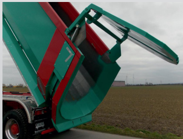
Hydraulic tailgate with large opening
