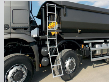
Access ladder with platform
