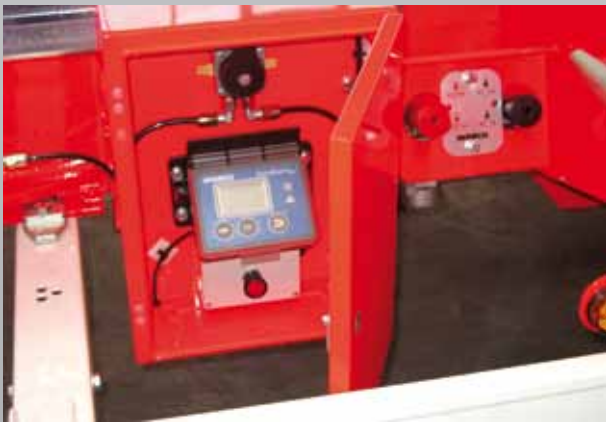
Function switch in protective box
