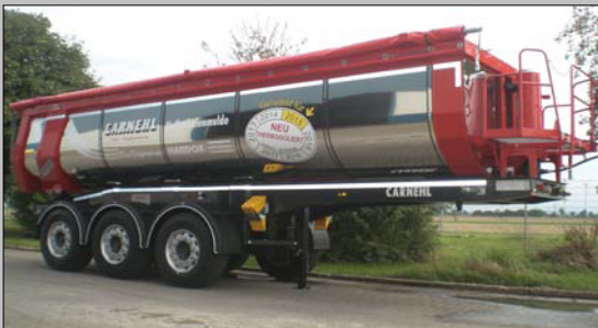
Insulated half-pipe dump body
