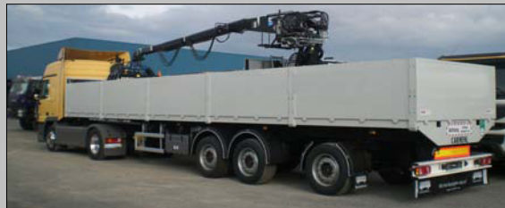
Building-material semitrailer with roller crane
