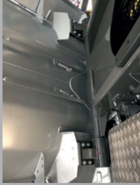
Wide-spaced rear body mounts
