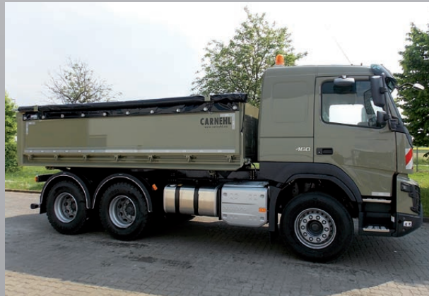
3-way tipper body with aluminium sidewalls
